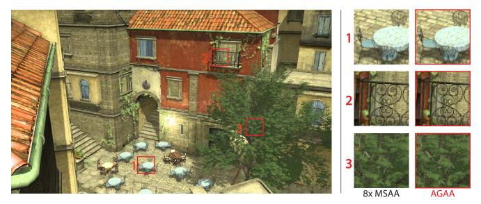
**Figure 1:** Large image rendered with Aggregate G-Buffer Anti-Aliasing (AGAA). The AGAA results (red outlines) shaded only twice per pixel give comparable results to the MSAA reference shaded eight times per pixel, and use 37% less memory. AGAA reduces aliasing by prefiltering the scene's sub-pixel geometric detail (foliage, thin railings, etc.) into a small set of statistical aggregates per-pixel.
